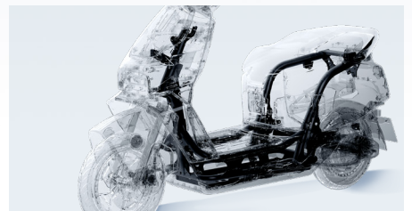
• Dual-arm fence frame for increased structural strength
